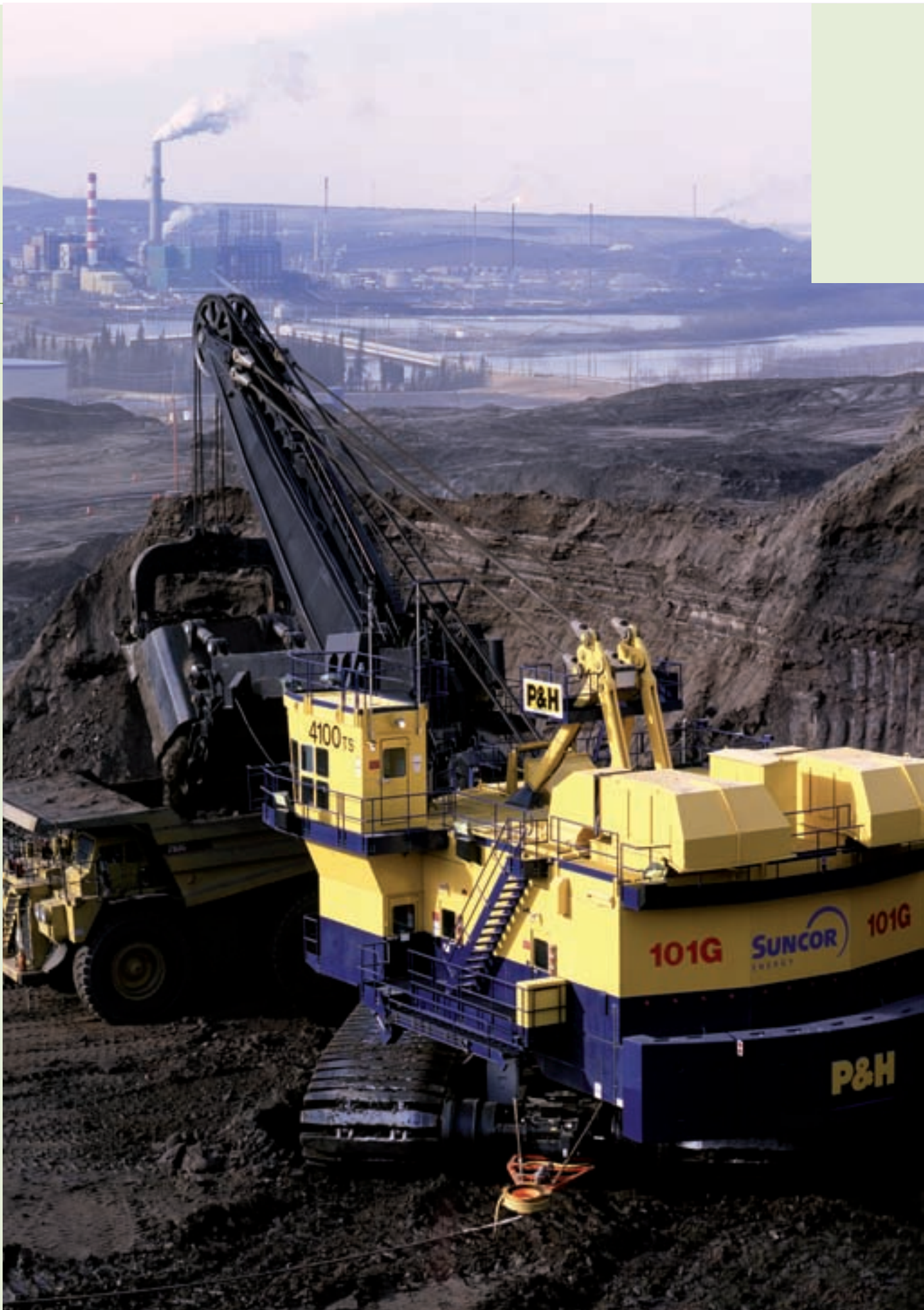
Shovels contain several ropes made of Bekaert wires: pendant lines, hoist ropes and trip ropes. Hoist ropes usually last a relatively short time. Together with our customer, we improved the ropes to prolong their life time.
