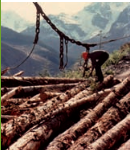
The hardware used to grab the logs consists of wire rope logging chokers, made from Bekaert high carbon wire, that are wrapped around the logs for transportation. ↑
